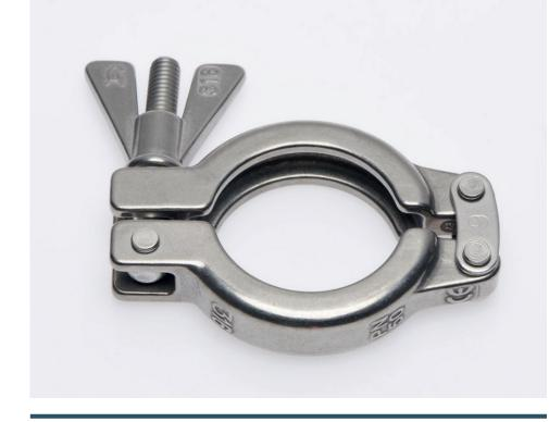
The SH Safety Clamp is based on the design of the widely accepted 316 stainless steel SH clamp, which includes the 'Omega' internal profile geometry known for its exceptional clamping efficiency. The SH style Safety Clamp's unique feature is the lower portion of the bolt is wider than the opening in the clamp's gate. In use, the wing nut must be deliberately loosened so the clamp gate can be lifted above the wider part of the bolt before the clamp can be completely opened.
