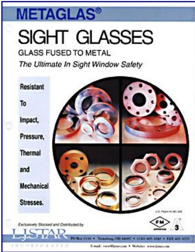
A new brochure from L.J. Star describes its line of ultra-safe prestressed Metaglas® sight glasses. Made by fusing pure borosilicate glass within stainless steel rings the result is a sight glass that has been described as having the transparency of glass with the strength of steel.
