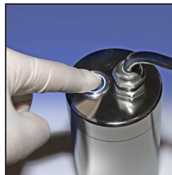
LumiStar2000 USL 15/35 with programmable on/off switch.
